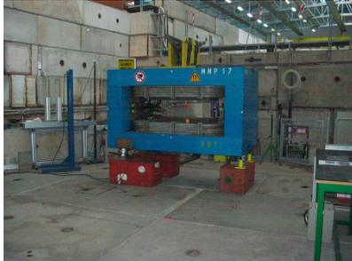
CERN's large, polarity-changeable, horizontal dipole magnet has a maximum field of 0.96 T over a length of 52cm. The gap height is 30 cm and the useful aperture width is 1m. The field can be varied by adjusting the current. This magnet can be installed inside the experimental area on request in order to determine the momentum of the particles.
